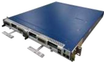
The DCI transmission and OLS capabilities of the Coriant Groove™ Open Line Solution can be combined to create high-density stackable solutions. For example, 96 carriers originating from 12 Groove G30 DCI elements can be multiplexed and amplified with a single Groove G30 OLS node. Components of the stackable solution can be deployed simultaneously or incrementally as DWDM capacity is required.
